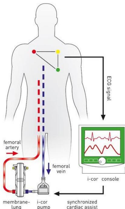
**The i-cor Synchronized Cardiac Assist System is the world's first circulatory support system to pump in synchrony with the heart and designed to: (1) improve coronary blood flow; (2) improve myocardial protection; (3) enhance organ perfusion.**
